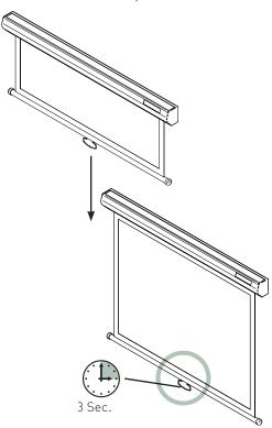
Retract the screen by pulling down the handle and then let go of it. The screen will retract into the casing.
